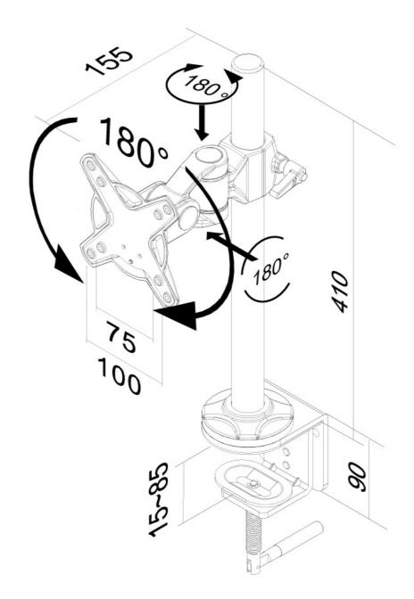
Neomounts Measuring unit: mm
