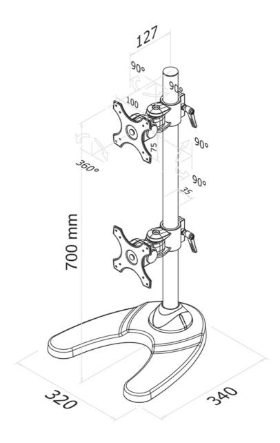
Neomounts Measuring unit: mm
