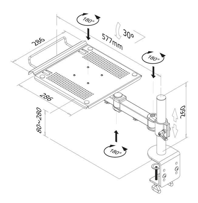
Neomounts Measuring unit: mm
