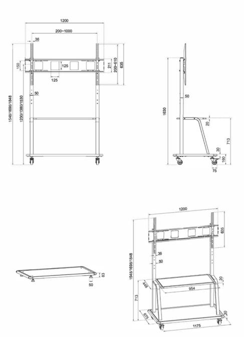
Neomounts Measuring unit: mm
