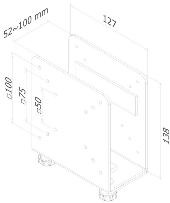
Neomounts Measuring unit: mm
