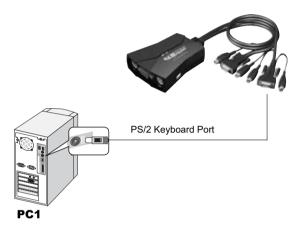
3. Connect the PS/2 mouse cable that is built into the KVM cable of your switch to the PS/2 mouse port on your computer.
