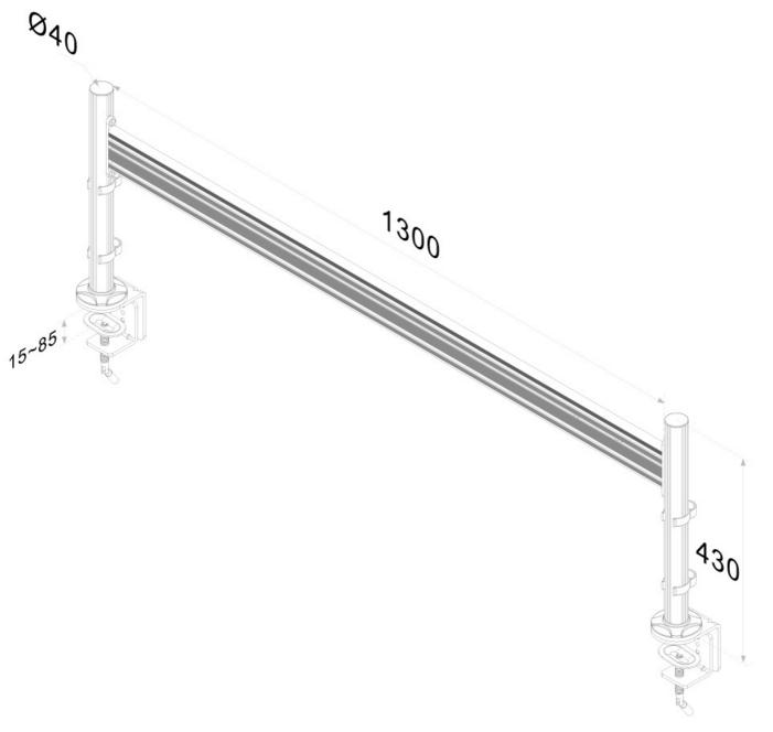
Neomounts Measuring unit: mm
