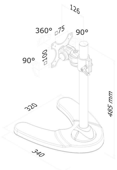
Neomounts Measuring unit: mm
