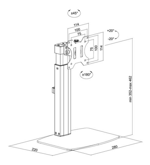
Neomounts Measuring unit: mm
