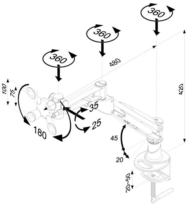
Neomounts Measuring unit: mm
