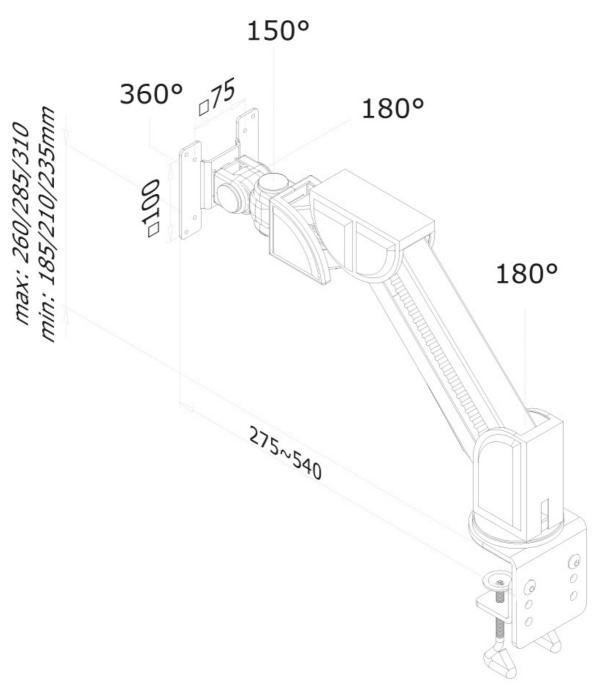
Neomounts Measuring unit: mm
