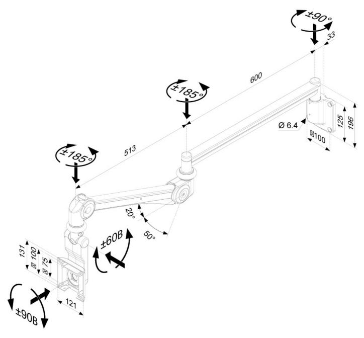
Neomounts Measuring unit: mm
