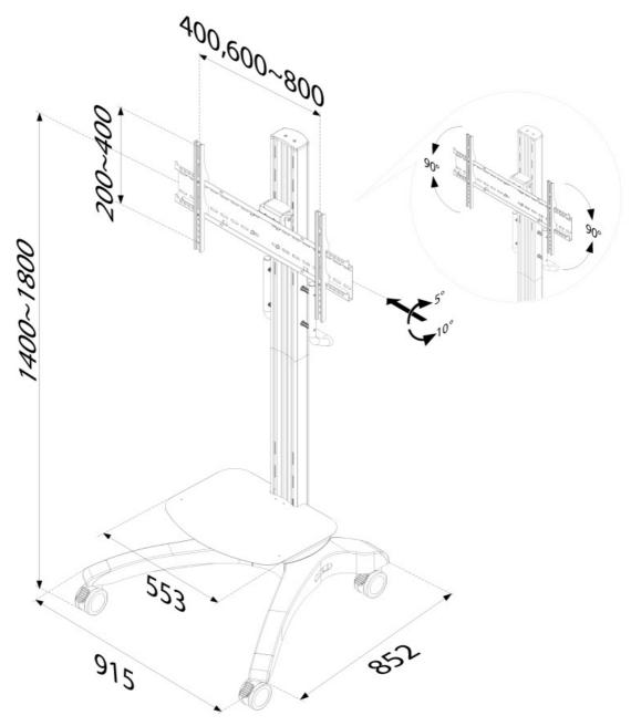
Neomounts Measuring unit: mm
