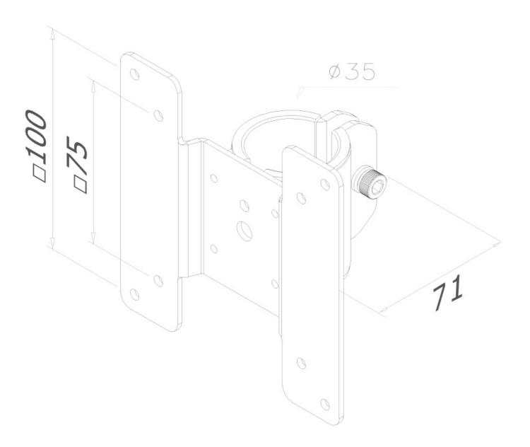
Neomounts Measuring unit: mm
